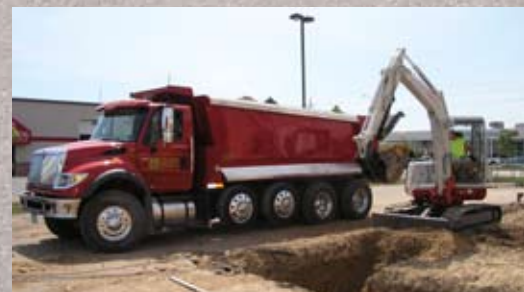
A Takeuchi mini-excavator is used for additions, remodeling projects, small excavation, and new construction.
